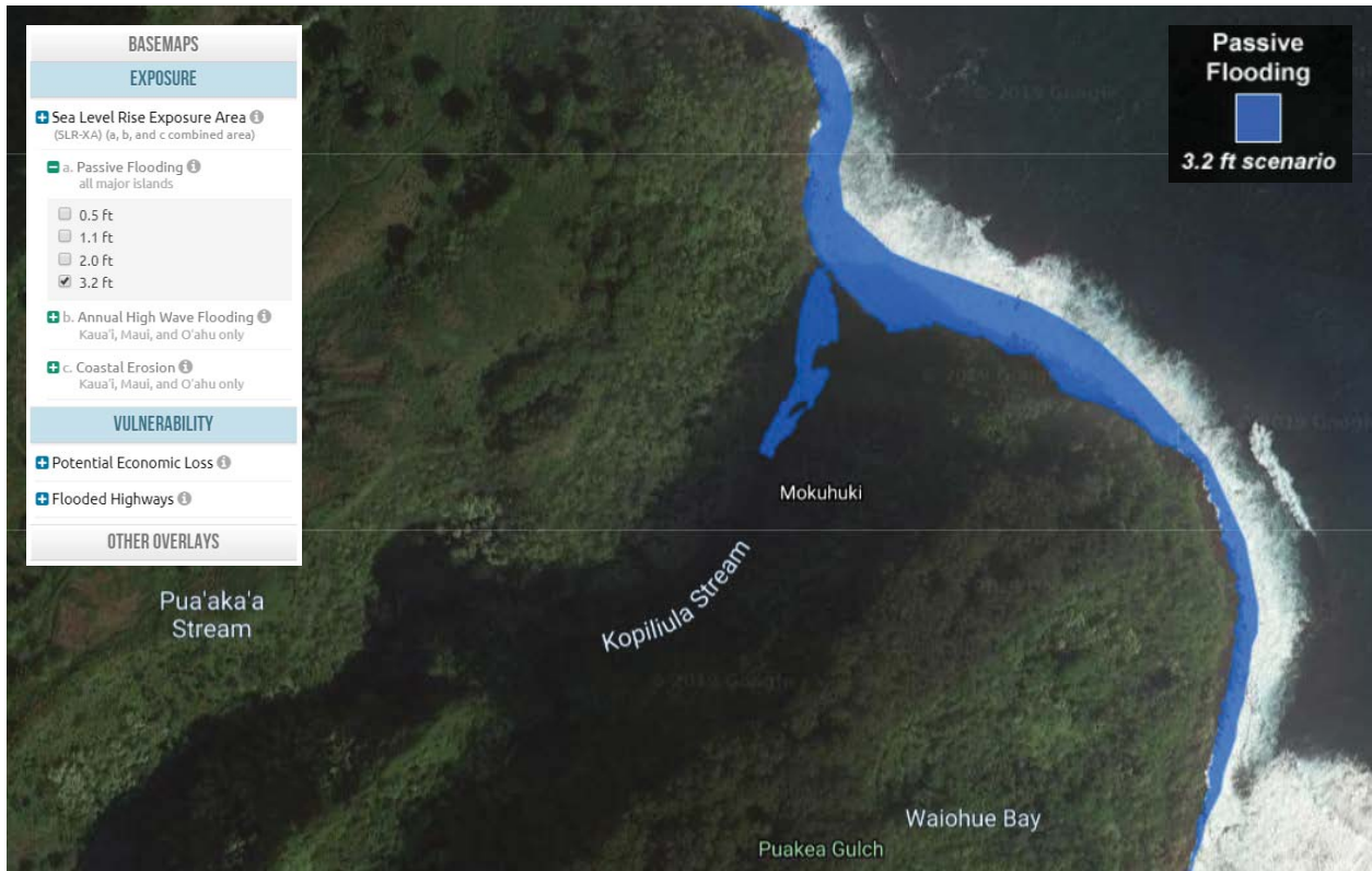
Figure 2-8. PacIOOS +3.2 ft sea level rise passive flooding projection Kopiliula Stream
