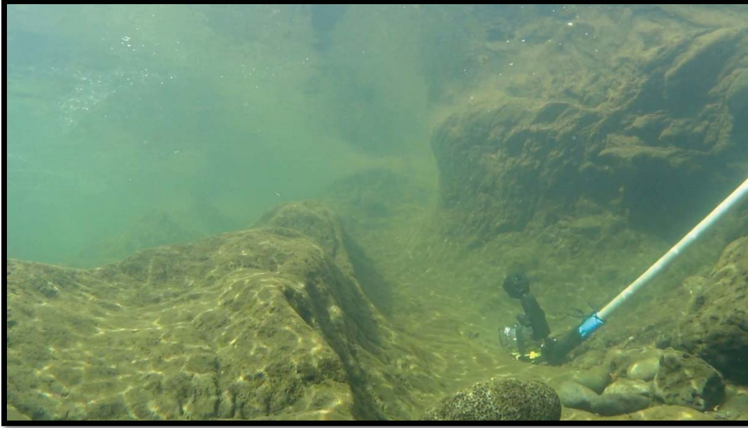
Figure 6: Underwater geo-referenced video camera with external video light used for the HDFS observations.
